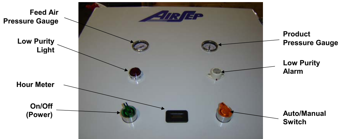
Figure 4.2: PSA Enclosure Controls and Indicators
