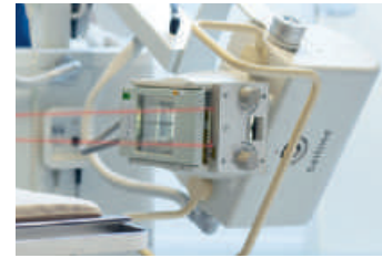
The fixed SID laser light option shows the Source to Image position at 100 cm to allow quick positioning
