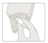
Place microcuvette into analyzer.
