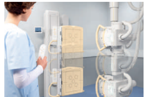
Tube Tracking at the fixed vertical stand VS
