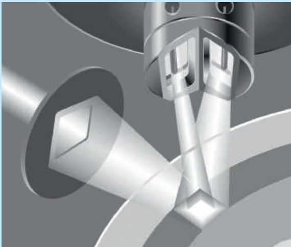
Principle of the "mixed" focus spot, here with a diagram
